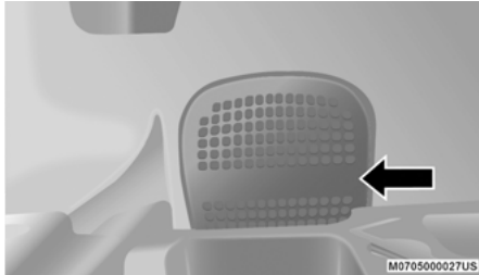
Rear Fuse Panel
