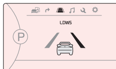
When the LDWS sensor detects the vehicle veering outside of the lane traveling in, a yellow indicator will illuminate
