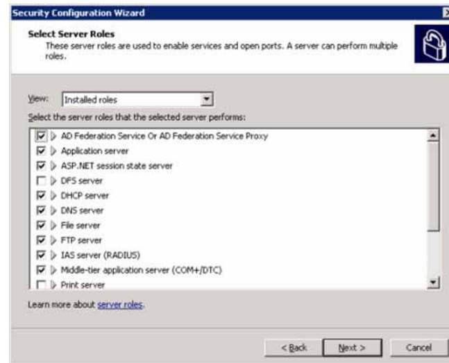
Figure 68 Role-based service configuration - installed roles
