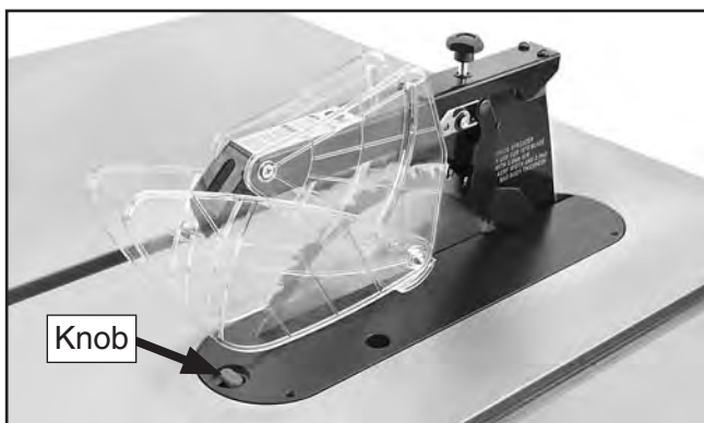
Figure 50. Blade guard and insert installed.
