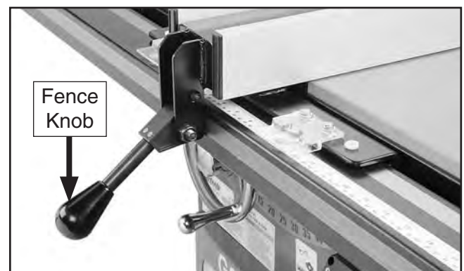
Figure 29. Fence knob installed.
