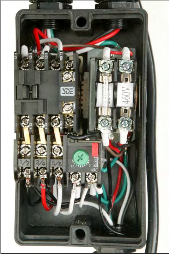
Figure 152. G0652 magnetic switch prewired to 220V, 3-phase.
