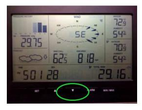
To tell the weather station to start communicating with the software, press and hold the button showing a down arrow until the weather station beeps (approximately 3-4 seconds).
