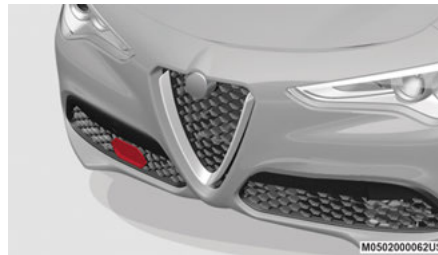
Front Bumper Radar Location
