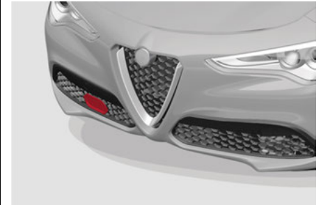
Front Bumper Radar Location
