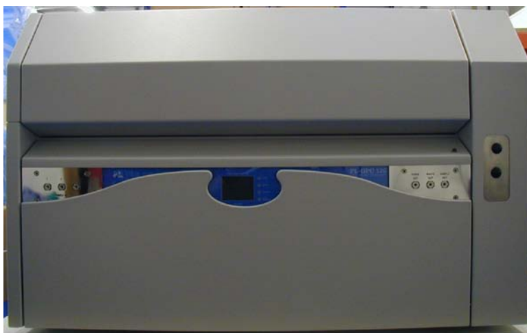
Mark II- extended end panel for installation of a Viscometer or Light scattering system
