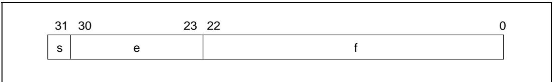
Figure 3.3 Floating-Point Number Format
