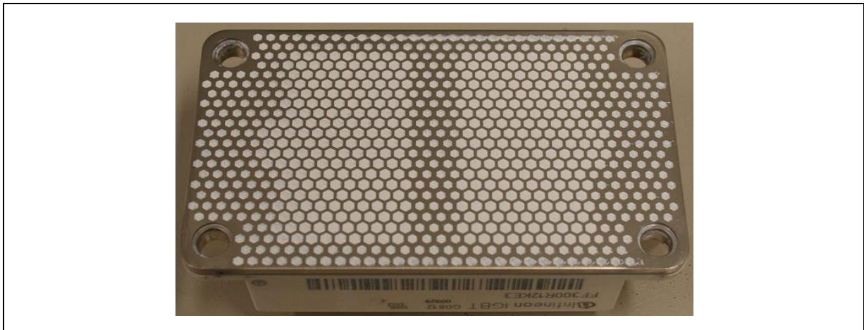
Fig. 6: 62mm module with IFX TIM
