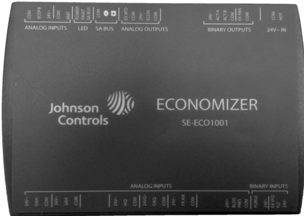
Figure 25: SE-ECO1001-1 Economizer Controller
