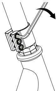
**1** Loosen the collar clamp and slide it upward. With a clock-wise twisting motion, push and "thread" the steer tube onto the fork until it bottoms out on the fork headset lock nut.
