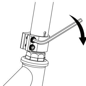
**1** Loosen the collar clamp and slide it upward. With a clock-wise twisting motion, push and "thread" the steer tube onto the fork until it bottoms out on the fork headset lock nut.
