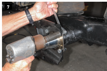
7) Install the Kodiak caliper flanges to the axle flange, torquing to the manufacturer's specifications. 8) During installation of the hub and rotor assembly, be careful not to damage the spindle or threads.
