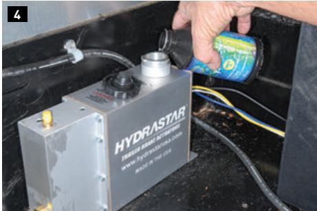
1) The HydraStar actuator employs a simple four-wire system using standard RV wire color code. 2 and 3) When installing the actuator in a storage compartment, be sure to use cable clamps to secure the brake lines to avoid any type of damage. 4) During the caliper bleeding process, it's important that the actuator does not run out of brake fluid. Air will enter the brake lines, and you will have to start over again. 5) When starting the bleeding process of the brake lines, always begin at the farthest caliper from the actuator. 6) Before installing the new hub and rotor assemblies, clean the spindle and inspect for flaws or damage. Replace any parts that may be compromised.
