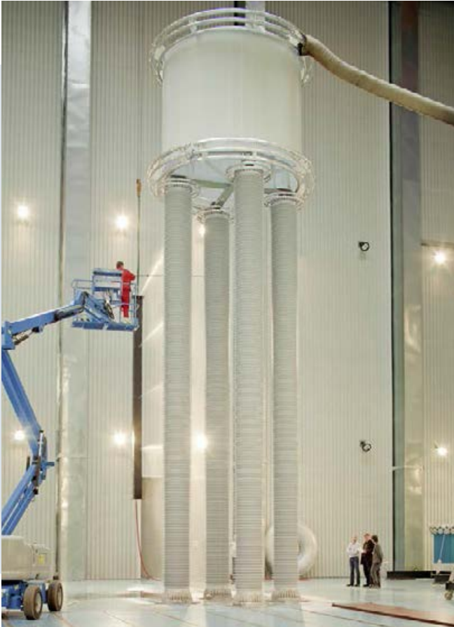
Fig. 68: Pole bus smoothing reactor for UHVDC Agra (BIL 1,300 kV; 2,680 A; 75 mH) – tests at HSP Cologne
