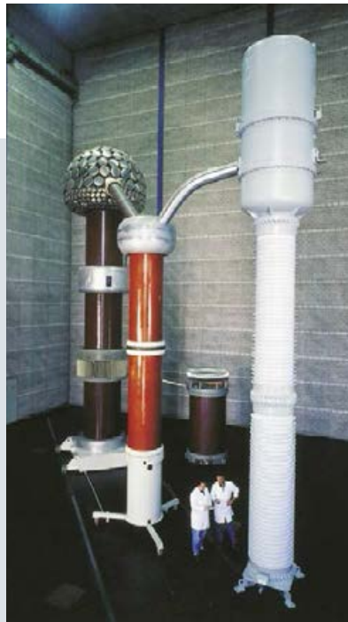
Fig. 51: 800 kV gas-insulated combined instrument transformers
