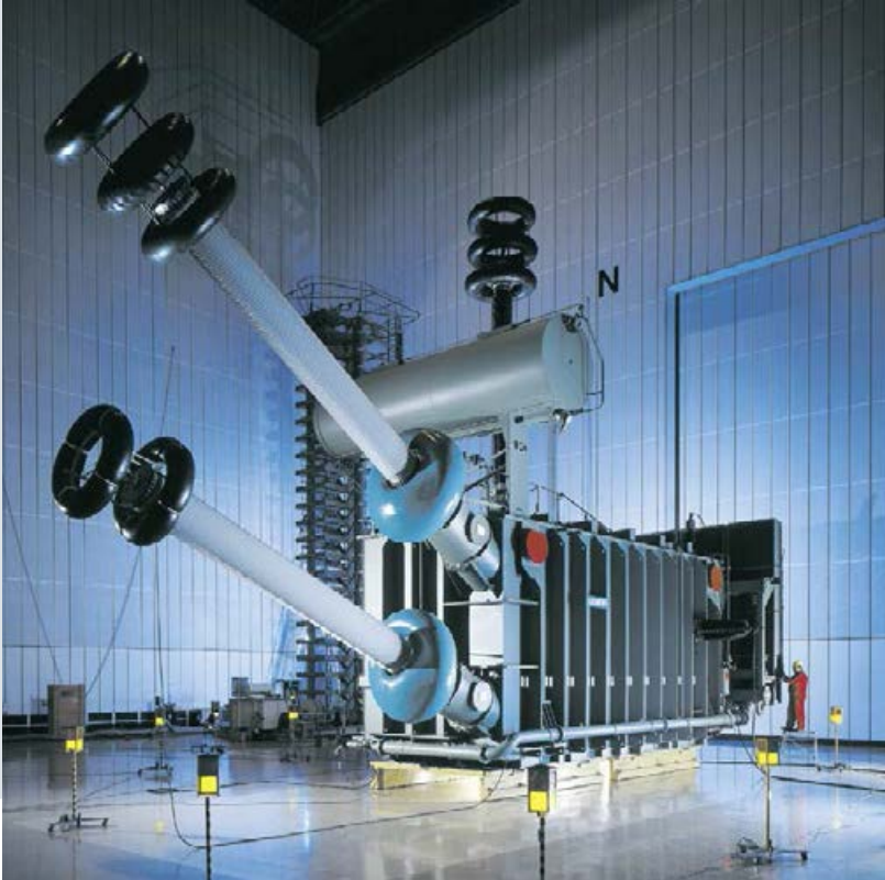
Fig. 80: Transformer bushing – 500 kV HVDC – project Three Gorges, China
