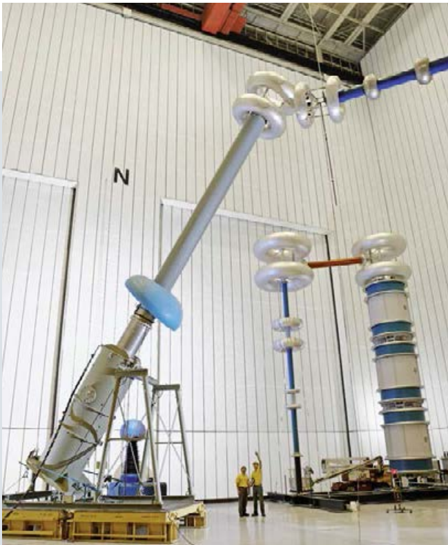
Fig. 77: Transformer bushing – 800 kV UHVDC – project Yunnan-Guangdong, China
