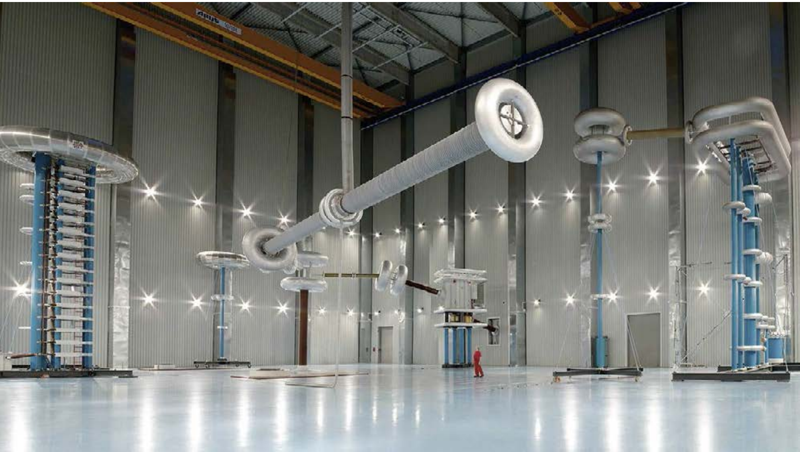
Fig. 78: Wall bushing – 800 kV HVDC – project Yunnan-Guangdong, China
