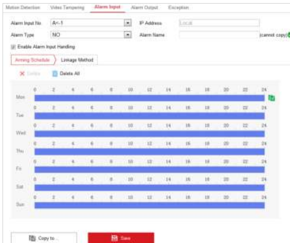
Figure 6-51 Alarm Input Settings
