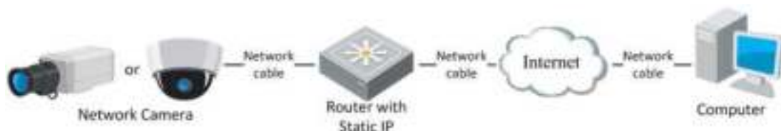
Figure 2-10 Accessing the Camera through Router with Static IP
