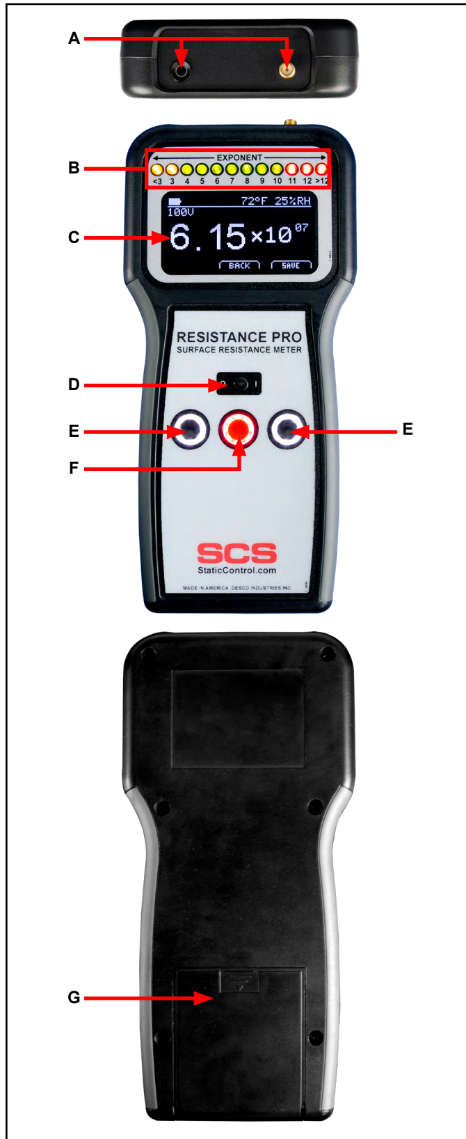
Figure 4. Resistance Pro Meter features and components
