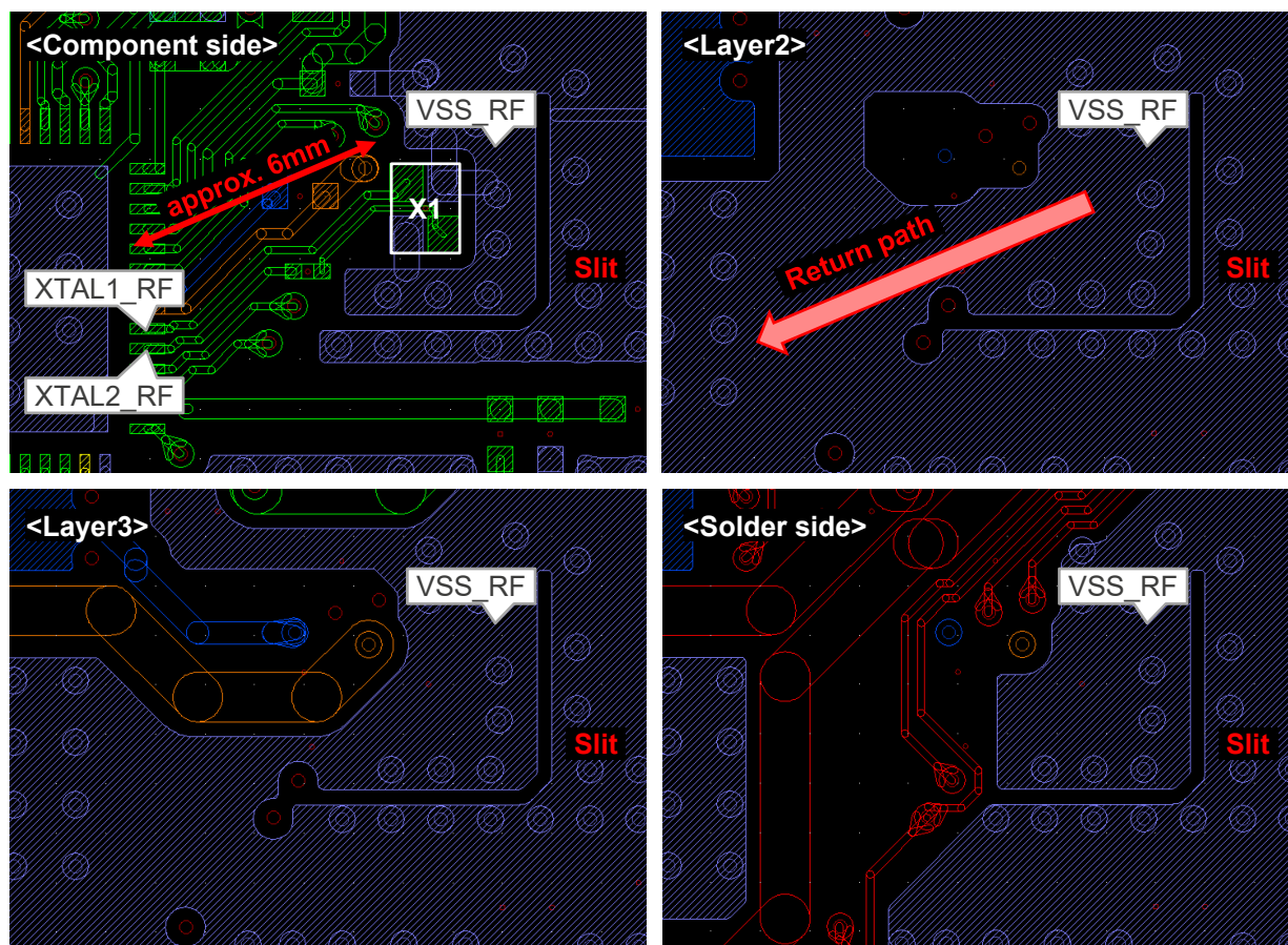
Figure 2-2. Example of the pattern around the crystal resonator
