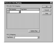
A Logix 5000™ controller stores tag names on the controller so that other devices can read or write data without having to know physical memory locations. Many products only understand PLC/SLC data tables, so the Logix 5000 controller offers a PLC/SLC mapping function that lets you map Logix tag names to memory locations.
