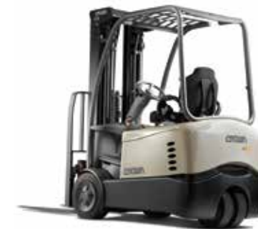
SC 5200 Series 3-Wheel Sit-Down Counterbalanced Truck Load Capacity: 3000 to 4000 lb Lift Height: 172 to 276 in
