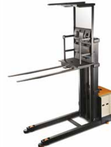
SP 3580F Series Platform and Cart Handler Voltage: 24 volts Load Capacity: 1500 lb Lift Height: 210 to 366 in
