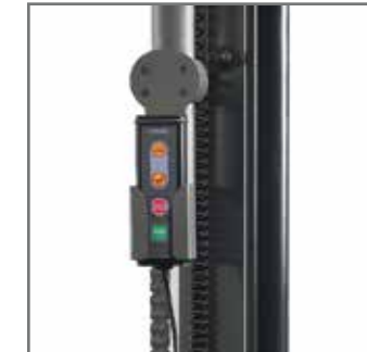
Remote raise/lower controls
