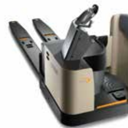
PR 4500 Series Side-Stance Rider Pallet Truck Load Capacity: 6000 and 8000 lb Double and triple fork length options are available
