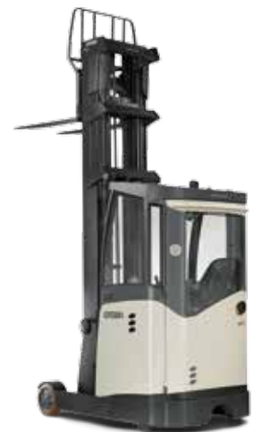
SR 5000 Series Mast-Moving Reach Truck Load Capacity: 4500 lb Lift Height: 163 to 450 in
