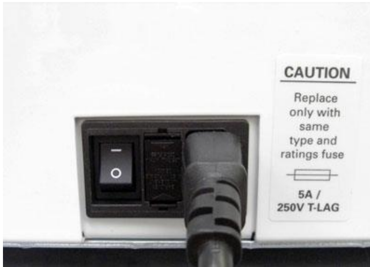
Shows the power switch in the back of the embosser
