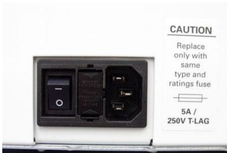
Shows the power module in the back of the embosser
