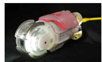
Underwater ROV for investigating inside the primary containment vessel of Unit 3
