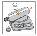
A completely full cartridge is an absolute prerequisite for the proper functioning of the ABS Avalanche Airbag.
