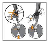
Only then is the handle attached properly and ready to use. If the handle will not attach refer to point 12.1. If the handle is not attached properly and is stuck due to the coupler snapping back into place, a proper activation will be impossible.
