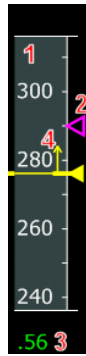
The current airspeed is 276 knots (Mach 0.56) and the target speed is 290 knots (managed).
