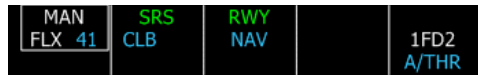
Typical FMA display when take off power is applied. The first column shows FLEX power is selected, and column 5 shows the autothrust system is armed.
