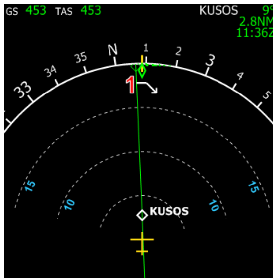
The top of descent point, computed by the FMGC, is shown with a white down arrow (1)
