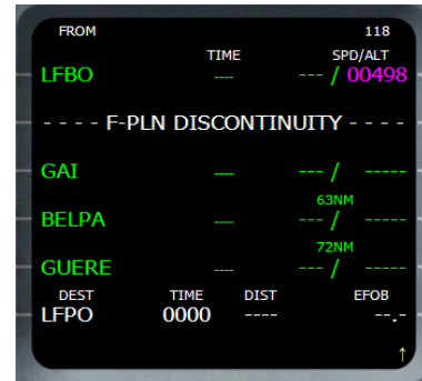
The route waypoints are added in the flight plan with discontinuities after departure and before arrival.
