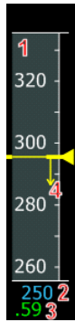
The current airspeed is 296 knots (Mach 0.59) and the target speed is 250 knots (selected).
