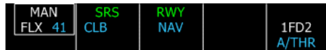
Typical FMA display when take off power is applied. Column 3 shows the runway mode is engaged (green RWY), and the NAV mode is armed (blue NAV).
