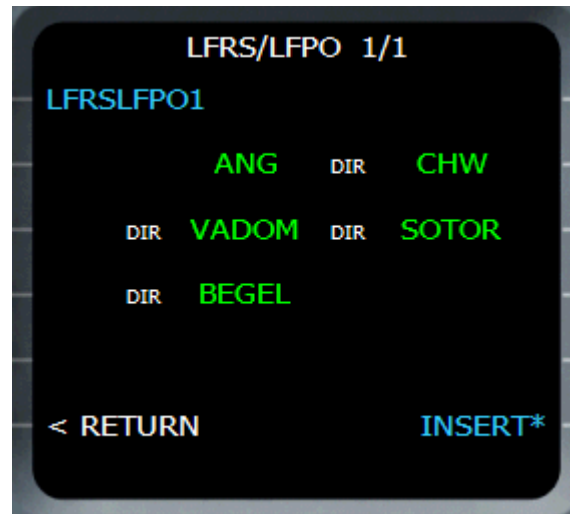
A route exists between LFRS and LFPO. You can use it by pressing INSERT (6R), or ignore it by pressing RETURN (6L).
