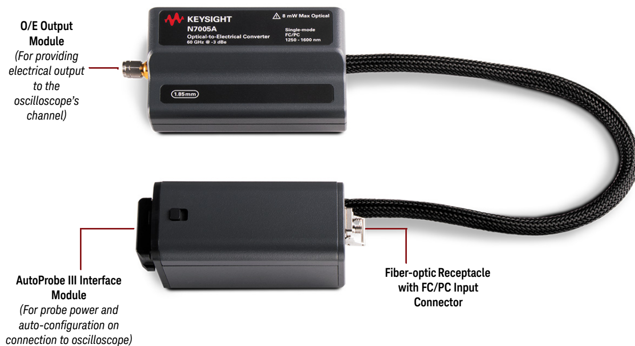
Figure 2 N7005A Optical-to-Electrical Converter - Components
