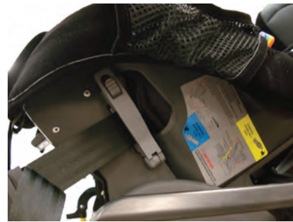
Figure 32 – Rear facing lock-off
