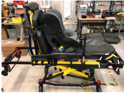
Figure 30 – Attach to the foot end extension tube
