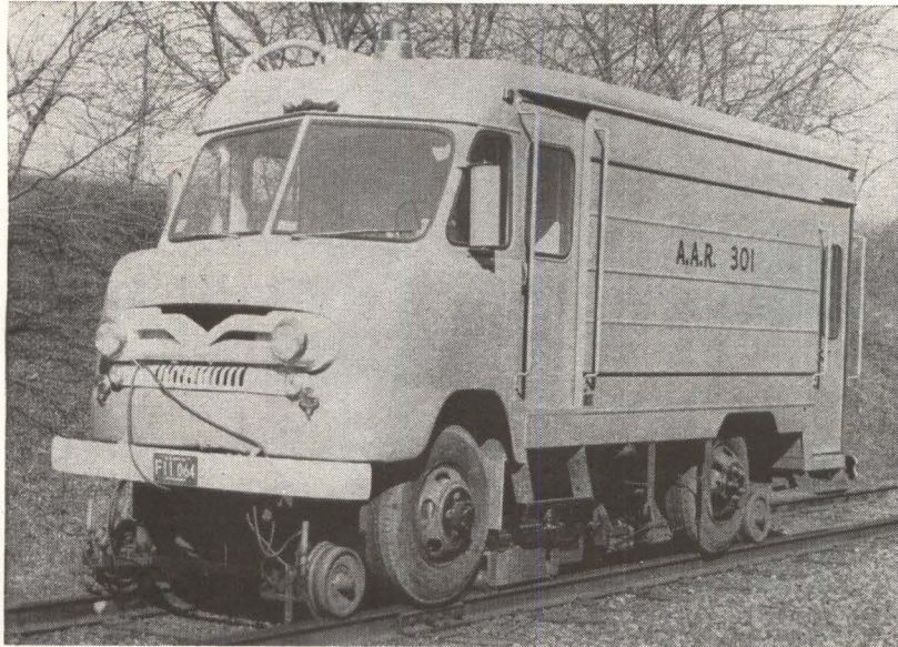
Road-rail trucks generally carry 12 amplifiers to obtain data on rail condition
