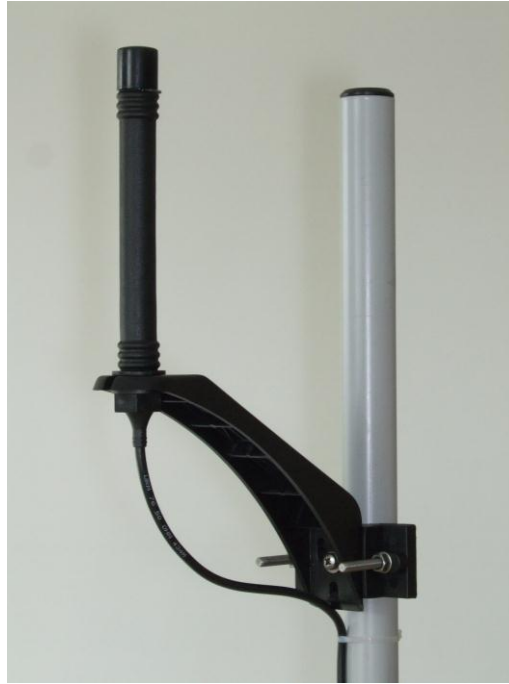
Figure 2 'Low-cost' dual-band antenna supplied by Campbell Scientific
