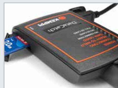
DataCatch device enables data collection
