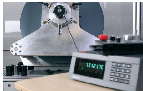
Rotational angle calibration system for direct and indirect measurement systems.
