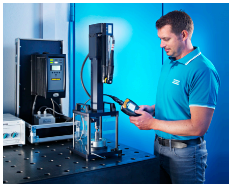
Calibration of a press tool system performed in a laboratory
