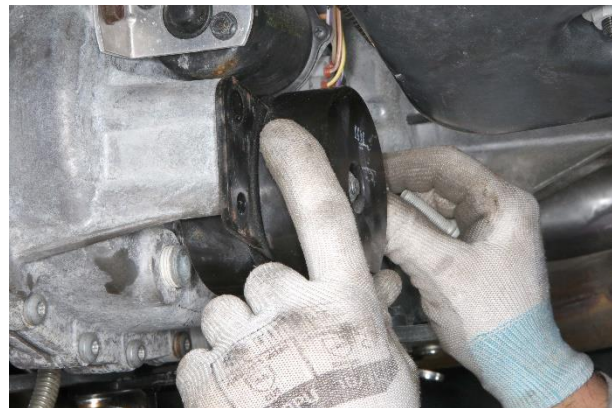
Figure 8 – Transfer Case Damper
