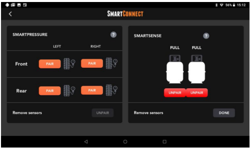
Figure 14: Unpairing SmartSense Propane sensor
