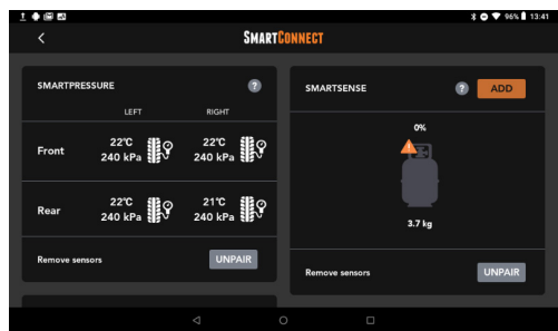
Figure 17: SmartPressure sensors icons after successful pairing
