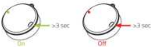
Figure 22: Instructions to turn on/off the SmartTemp Sensor
