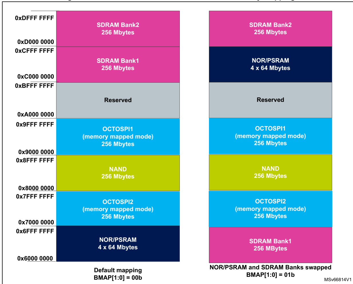
Figure 5. STM32H72x and STM32H73x external memory mapping
