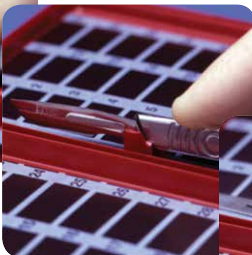
Step 2: Slide forward until blade "catches."
