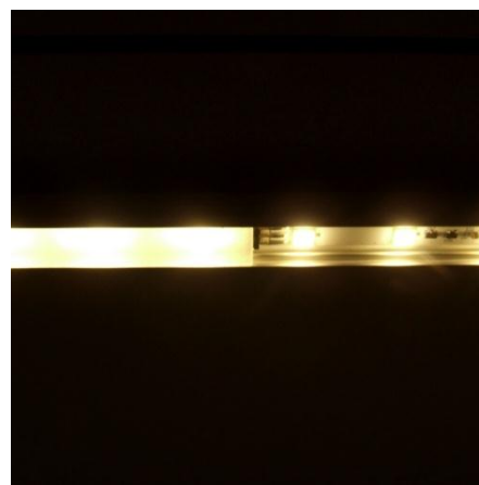
Diffuser applied on left half
