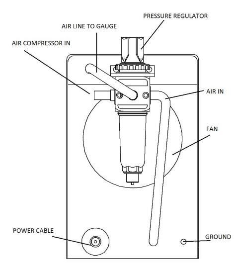
**AIR REGULATOR** – Apply supplied thread tape on all fitting, double check for any leaks
