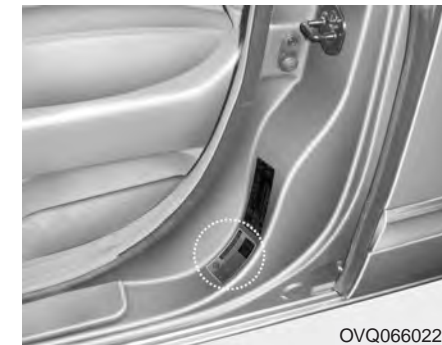
Tire specification / pressure label
