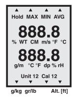
Alt. (ft) label on the case. Select with  $\blacktriangleright$ . Move the wheel up and down to adjust the altitude. You can select with  $\blacktriangle$  and  $\blacktriangledown$ ; confirm by  $\blacktriangleright$ .
