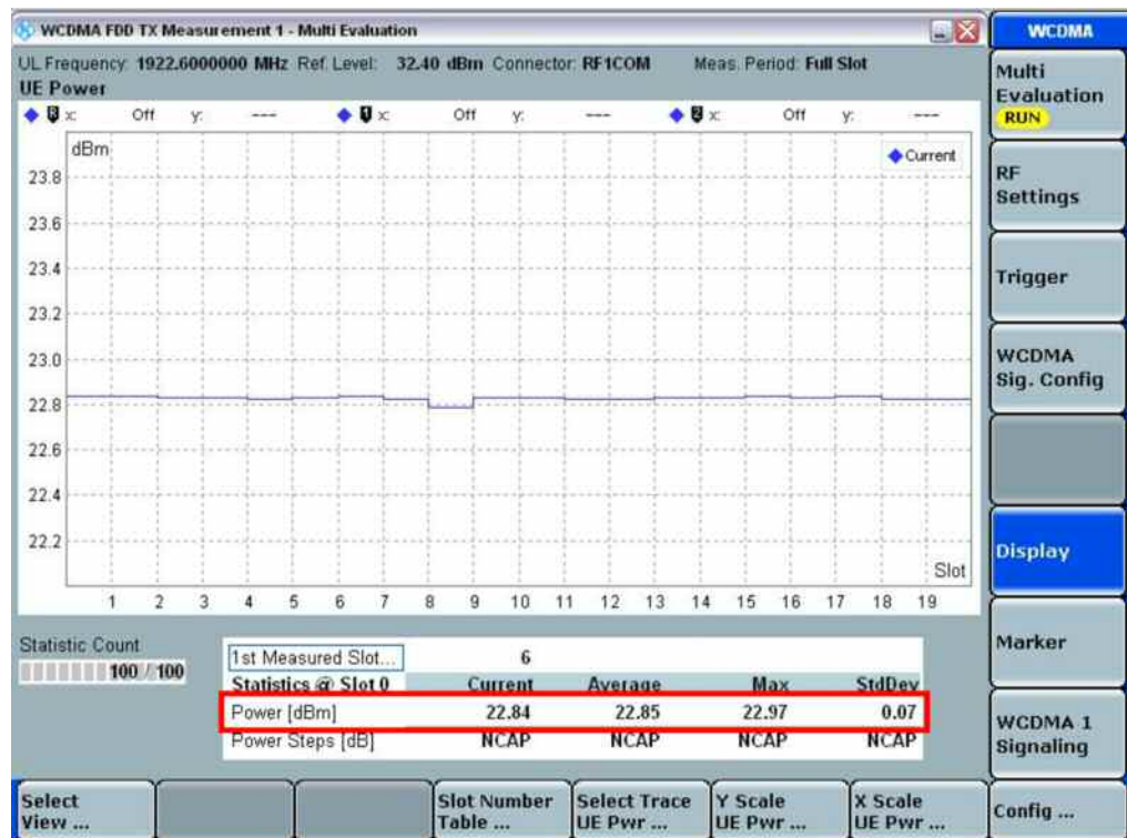
Fig. 9: Results from a maximum output power measurement.
