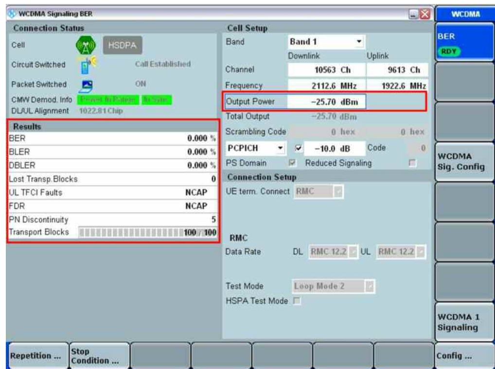
Fig. 40: BER results for the maximum input level.
