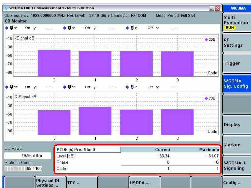
Fig. 25: Peak code domain error result for UE transmitting at its maximum power.
