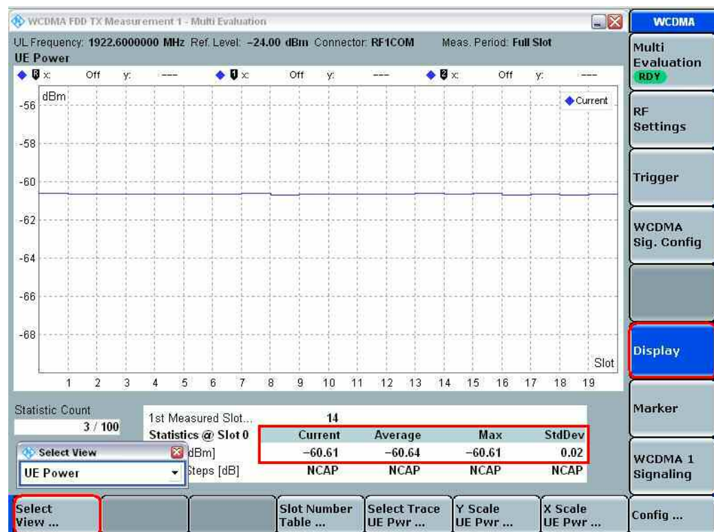
Fig. 15: Minimum output power measurement results.
