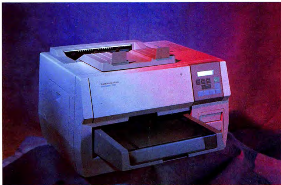
The Texas Instruments OmniLaser 2108 has the densest blacks of any unit tested. That's because it uses a Ricoh write-white engine. Unfortunately, the dense blacks sometimes lead to toner scatter in areas that should be white.
