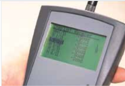
Checking signal strengths with hand held tool. Boost any poor signals with the router
