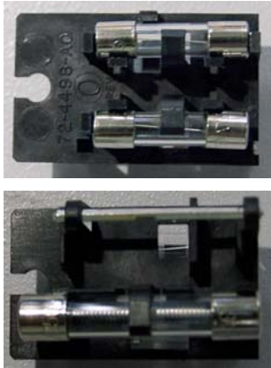
Figure 24 120 V fuse in holder
