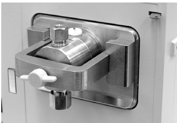
Figure 4 Pump head installed on the pump
