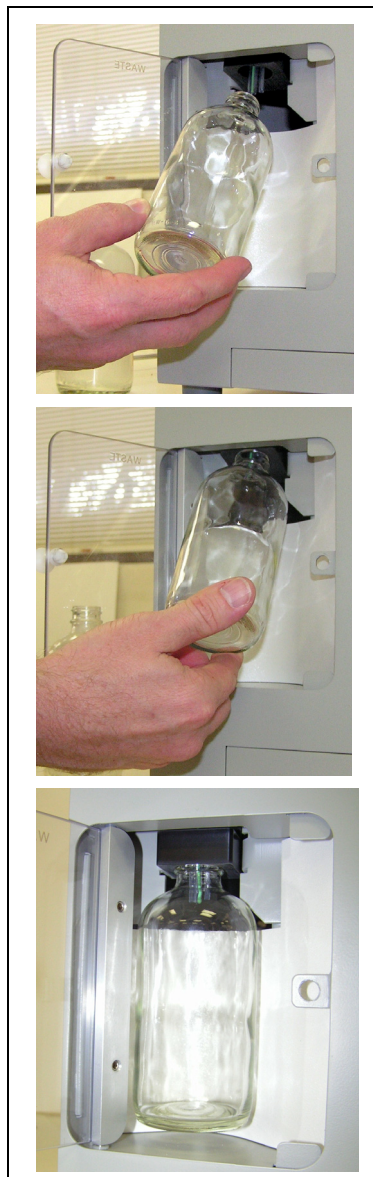
Figure 3-11. Installing the Waste Bottle
