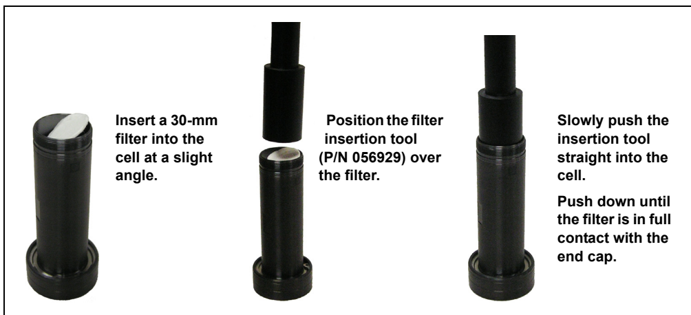
Figure 3-5. Installing a 30-mm Cell Filter in a 34-, 66-, or 100-mL Cell
