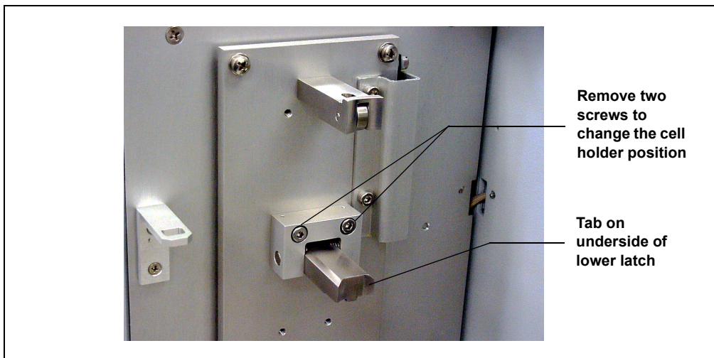
Figure B-7. Removing the Cell Holder Lower Latch
