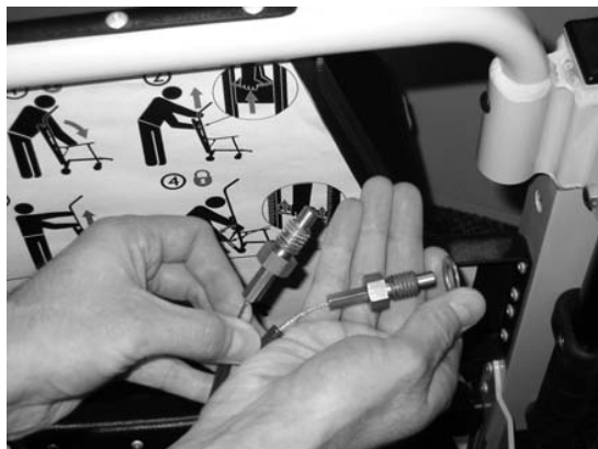
Figure 51: Place the washer on the new cable
