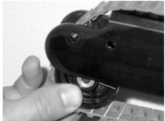
Figure 43: Remove the wheel spacer in the direction of the floor
