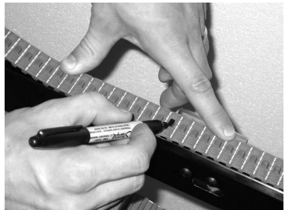
Figure 44: Mark a belt tooth for reference
