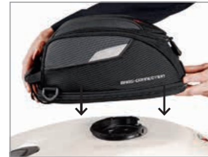
Lower the bag onto the EVO tank ring and press down to engage
