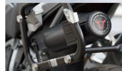
Tool tube box (30 x 9 x 11 cm) mounted on the inside of QUICK-LOCK EVO side carrier.
