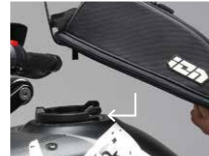
Lower the bag from behind the tank ring
