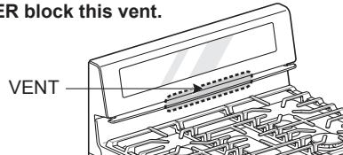
**Do not cover the cooktop surface with aluminum foil. Blocking the oven vent can damage the control panel.**
