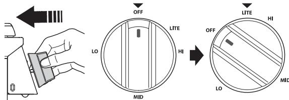
The electric spark ignition system makes a clicking noise. Once the burner is lit, turn the knob counterclockwise to the **HI** position to stop hearing the clicking noise.
