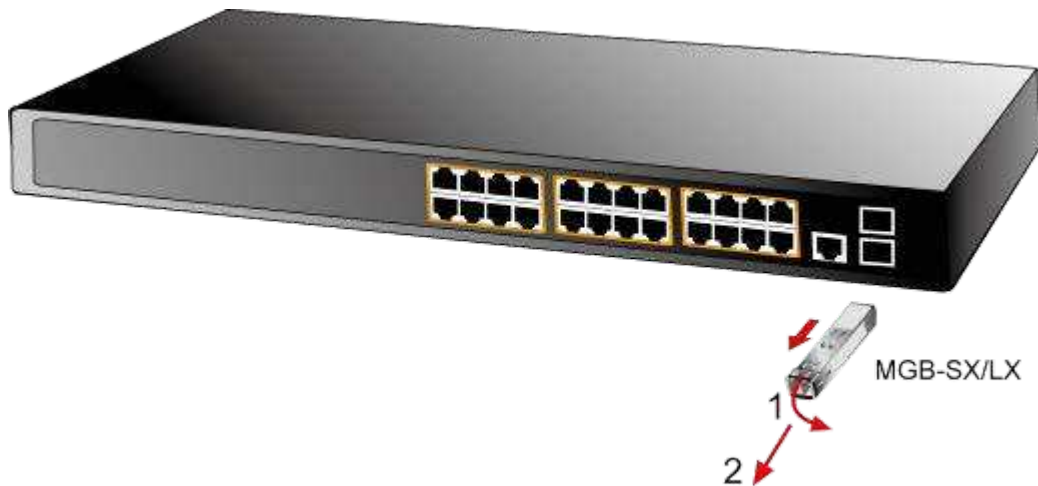
Figure 2-1-13: How to Pull Out the SFP Transceiver
