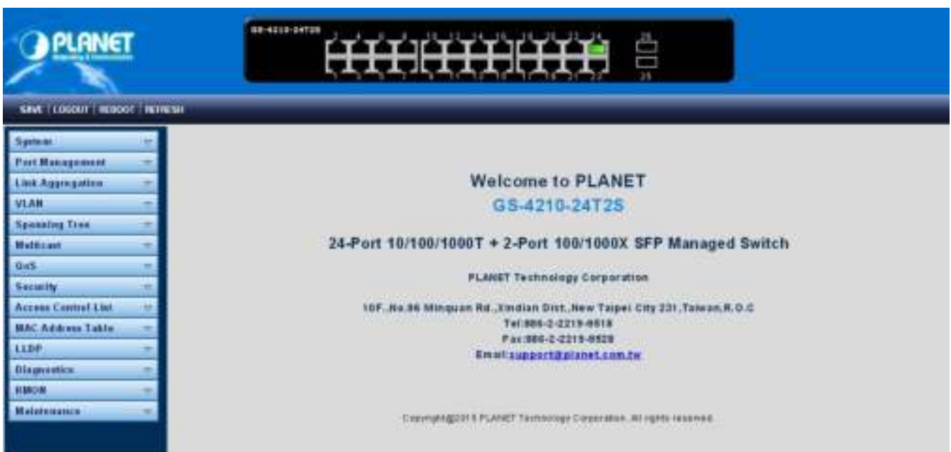
Figure 4-1-3: Web Main Screen of Managed Switch
