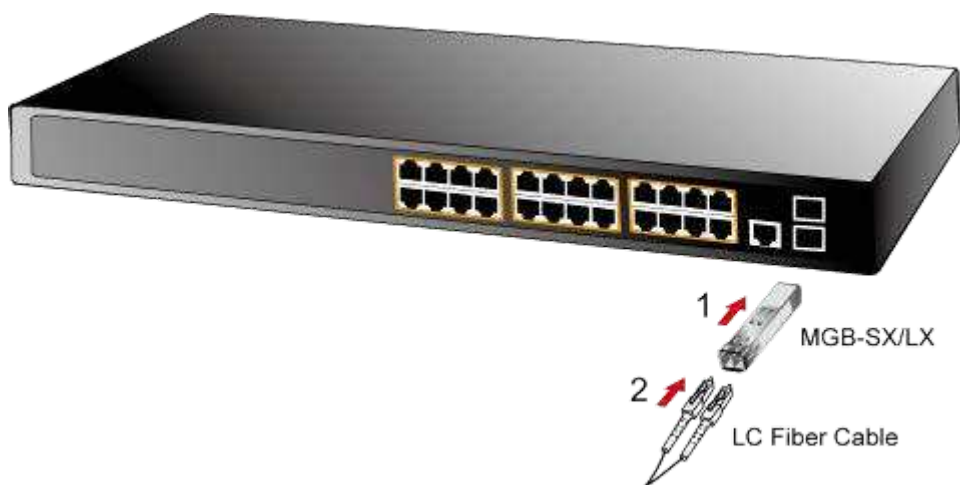
Figure 2-1-12: Plug In the SFP Transceiver
