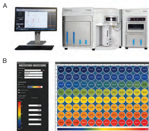
Figure 1. Setup of Attune NxT Flow Cytometer with Autosampler for high-throughput screening experiments. (A) Invitrogen™ Attune™ NxT Flow Cytometer with Invitrogen™ Attune™ NxT Autosampler. (B) Plate heat-mapping is available on Invitrogen™ Attune™ NxT Software to monitor results as they are acquired.
