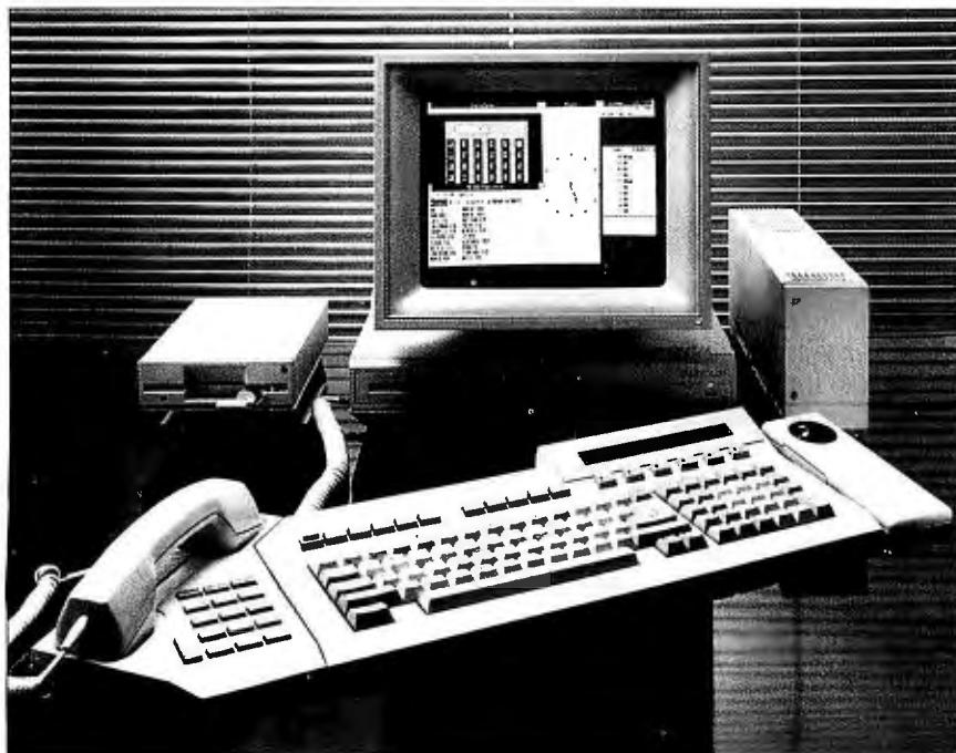
Photo 1: The new Apricot XEN 80286-based business microcomputer. It is shown with a 360K-byte 5¼-inch floppy-disk unit and an expansion box, which can house up to two IBM expansion cards; these units provide some compatibility with the IBM PC and the PC AT. The optional combination trackball/mouse and telephone are also shown. The XEN is seen running Microsoft Windows, which is its standard operating environment.
