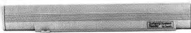
The Cauzin Softstrip System Reader replaces tedious typing by scanning the strip and reading it into your computer.
