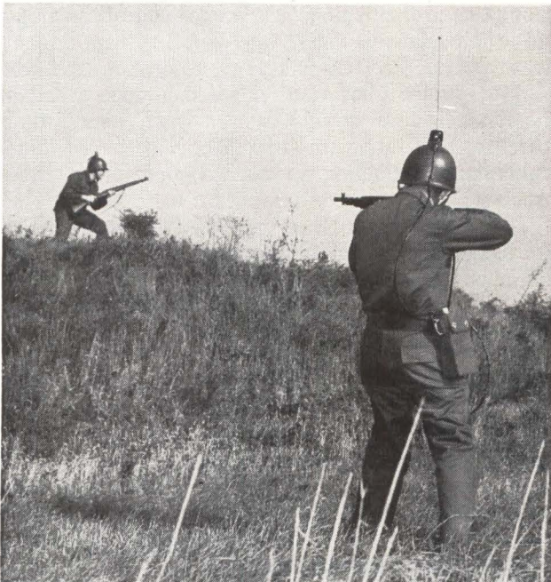
PHOTOELECTRIC telescope is attached to infantryman's rifle giving 500-meter range. Helmet mounts the combined quarter-wave antenna and beacon unit
