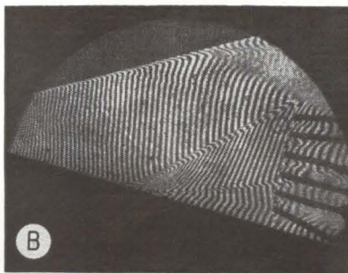
CONVENTIONAL interferogram, (A), was taken with filtered BH-6 mercury arc, air-to-air injection at Mach 2.3 station, 250 psi chamber pressure, 150 psi injection pressure. Laser interferogram (B) shows improved resolution, was taken with argon-to-air injection at Mach 2.3/station (point where flow reaches 2.3 Mach speed) 105 psi chamber pressure, 35 psi injection pressure
