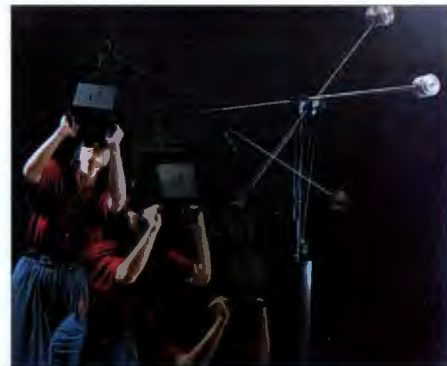
A NASA Ames researcher uses a Boom to look at data on computational fluid dynamics. Simulation software created on a Cray supercomputer by NASA processes the math. You can explore the data produced by the Cray by running Fakespace's interactive-virtual-environment application on a Silicon Graphics workstation.
