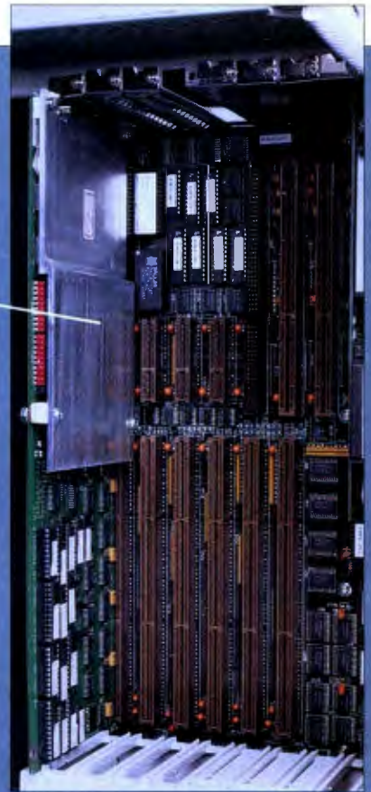
Acer took a unique approach to dissipating the heat generated by the Pentium in the AcerFrame 3000MP. A metal plate acts as a heat sink; it's thin enough to allow normal spacing of the expansion slots.
