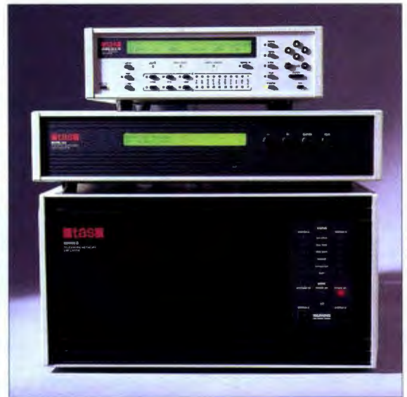
The TAS (Telecom Analysis Systems) Series II modem tester enabled us to re-create 25 telephone-line impairments; this helped us judge how well each modem worked under real-world conditions.
