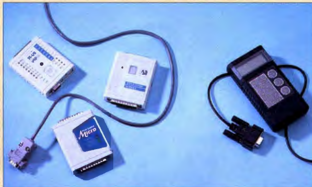
Blue Earth Research's Micro 440 (left) features a 12-MHz processor, eight 8-bit A/D channels, two serial ports, 32 KB of battery-backed RAM, a real-time clock, and 14 digital status and control lines. A customized version of BASIC runs the show. The Tattletale 5LCD runs off a Hitachi 6303 processor and comes with a serial port, digital I/O lines, EEPROM for storing program configurations, and a customized BASIC interpreter. As with the Micro 440, you connect the Tattletale to your personal computer and write your control program in BASIC or assembly language.
