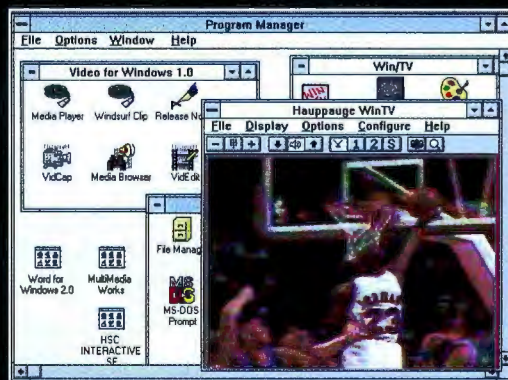
Resize or reposition your Win/TV window anywhere on the screen. The "always-in-front" mode allows the video image to always be viewable.
